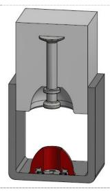
The MPB recess former with magnets is made of polyurethane resin and is used in combination with P anchor. These recess formers are mostly applied in an upside down position.
